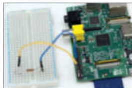
Fig 2: Place the female end onto the Pi, noting pin number 1 being identified by the small 'P1'. The blue wire is ground
