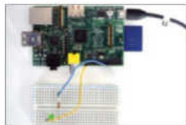
Fig 4: Switch the power on. The LED will light up. If it's dim, use a lower-rated resistor
